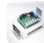
Optional CMB board for PWM fan, overheat & PSU alert functions
