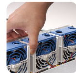
Easy-assembly fan bar with anti-vibration rubbers
