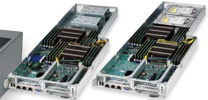
SYS-F617R2-FT+/FTPT+/F72+ 4x 2.5" HDDs per Node
