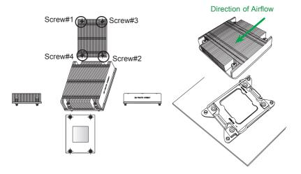
Note: For optimized airflow, please follow your chassis airflow direction to properly install the CPU heatsink. Graphic drawings included in this manual are for reference only. They might look different from the components installed in your system.
