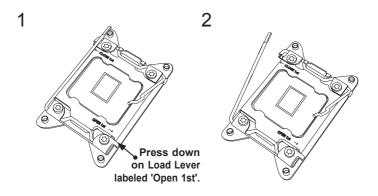
Note: Graphic drawings included in this manual are for reference only. They might look different from the components installed in your system. 2. Press the second load lever labeled 'Close 1st' to release the load plate that covers the CPU socket from its locking position.
