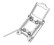
Warning: You can only install the CPU inside the socket in one direction. Make sure that it is properly inserted into the CPU socket before closing the load plate. If it doesn't close properly, do not force it as it may damage your CPU. Instead, open the load plate again and double-check that the CPU is aligned properly.
