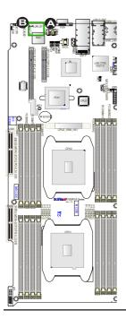
A. IB\_LINK\_LED1 (For X10DRT-PIBQ/ PIBF) B. IB\_ACT\_LED1 (For X10DRT-PIBQ/ PIBF) **Rear UID LED**
