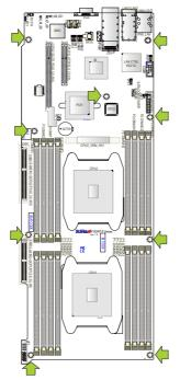
**Caution:** 1) To avoid damaging the motherboard and its components, please do not use a force greater than 8 lb/inch on each mounting screw during motherboard installation. 2) Some components are very close to the mounting holes. Please take precautionary measures to prevent damage to these components when installing the motherboard to the chassis.
