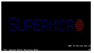
**Note:** On the other hand, if the following screen displays, please load the "Super.ROM" file to the root folder and connect this folder to the system. (You can do so by inserting a USB device that contains the new "Super. ROM" image to your machine for BIOS recovery.)
