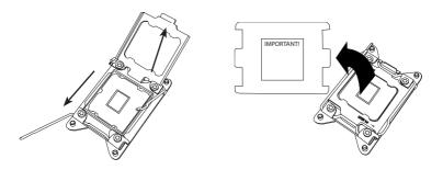
5. Use your thumb and index finger to hold the CPU on its edges. Align the CPU keys, which are semi-circle cutouts, against the socket keys.
