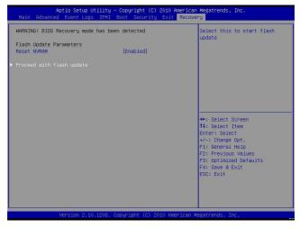
5. When the screen as shown above displays, using the arrow key, select the item "Proceed with flash update" and press the <Enter> key. You will see the progress of BIOS recovery as shown in the screen below.
