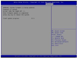
After the process of BIOS recovery is completed, press any key to reboot the system.
