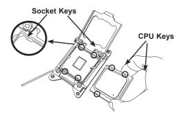
Once they are aligned, carefully lower the CPU straight down into the socket. (Do not drop the CPU on the socket. Do not move the CPU horizontally or vertically. Do not rub the CPU against the surface or against any pins of the socket to avoid damaging the CPU or the socket.)
