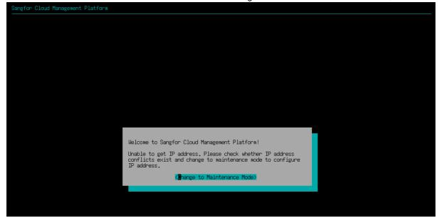
3. Click anywhere on the virtual machine console, type "enter" on the keyboard to enter maintenance mode, then enter the password (the initial password is admin), select the OK option after entering the password. Then type "enter" on the keyboard again to enter configuration interface.
