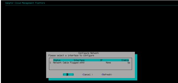
5. Configure IP address, netmask and gatewat and press OK.
