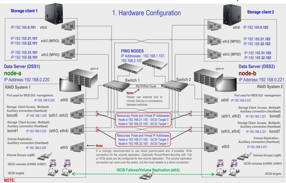
To prevent switching loops, it's recommended to use RSTP (802.1w) or Port Trunking on network switches used to build A-A Failover network topology.
