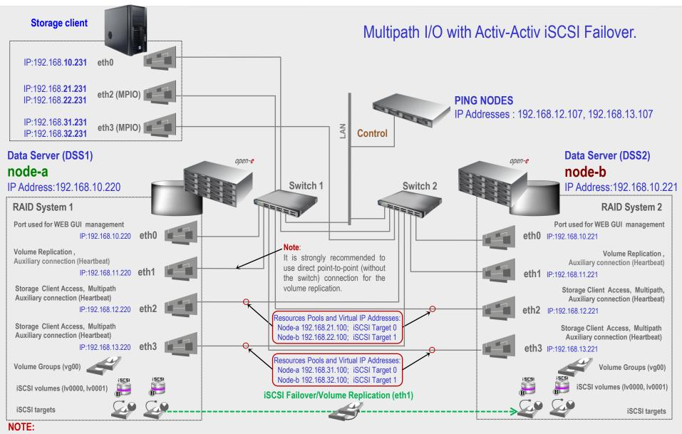
To prevent switching loops, it's recommended to use RSTP (802.1w) or STP (802.1d) protocol on network switches used to build A-A Failover network topology.
