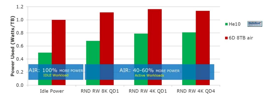
SIT Lab Testing (SATA) 10TB vs 8TB 6 Disk Comparison
