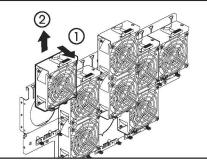
1. Moving the latch until hook releasing 2. Pull up fan module then fan board disconnecting.
